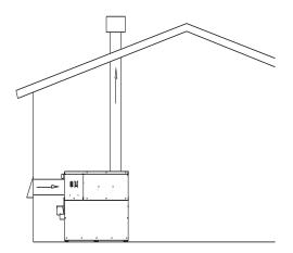
FIG. 14 Sidewall Combustion Air Inlet
